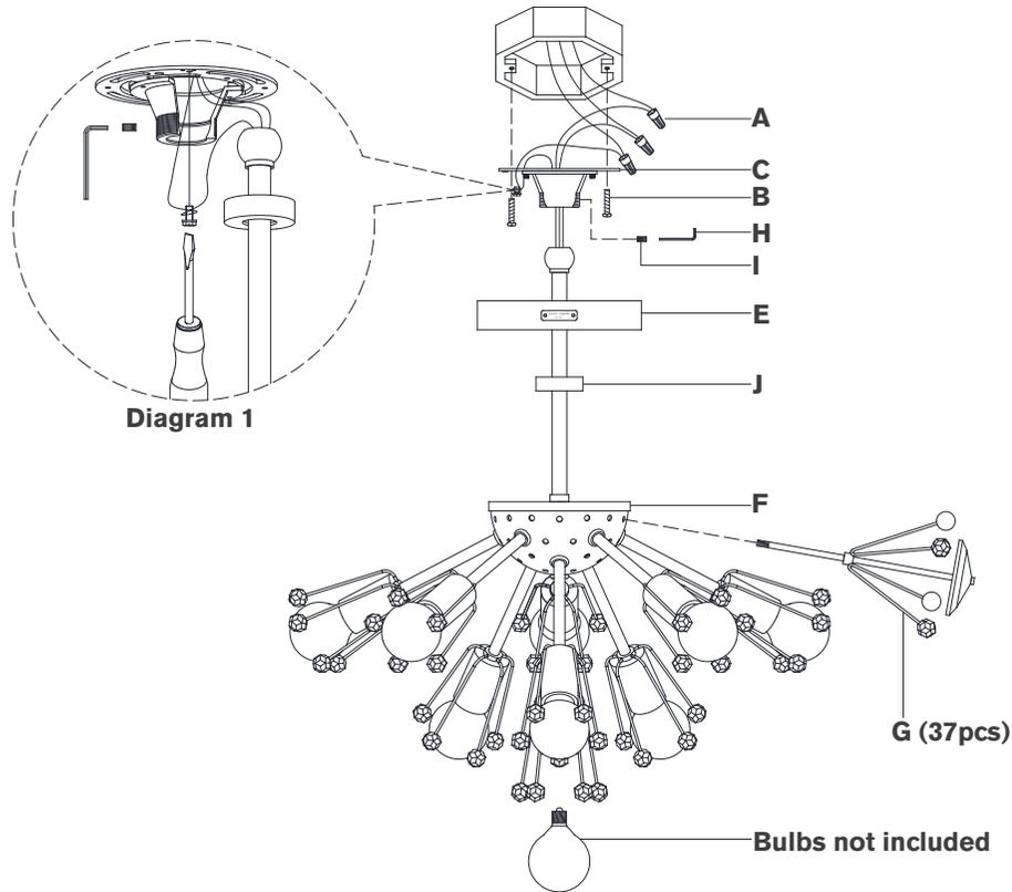
10. Install canopy (**E**) to mounting plate (**C**) by securing with collar ring (**J**).
